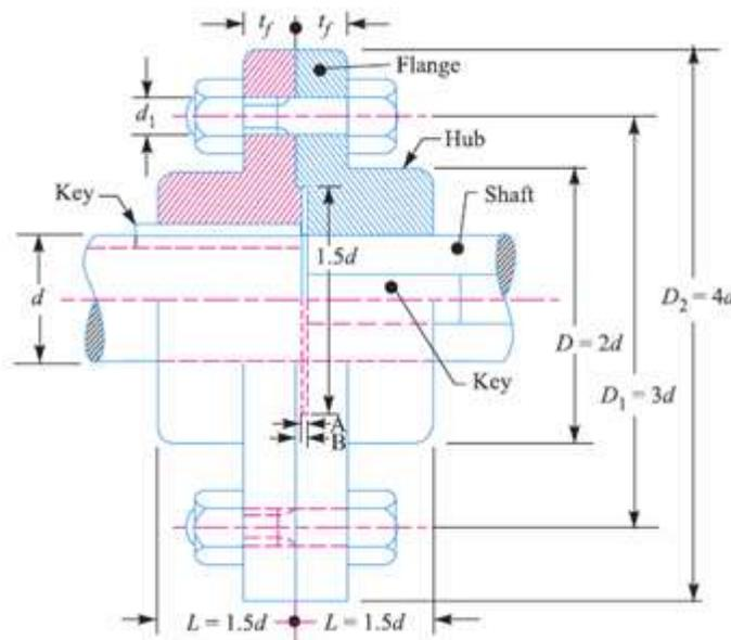
Figure 1.4 Flange Coupling
