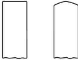
a. Flat Pulley    b. Crowned Pulley
