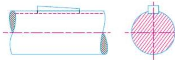
Figure 1 Rectangular Sunk Key
