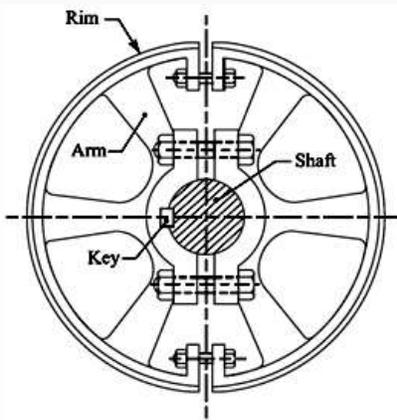
Figure:2 Split Cast Iron Pulley
