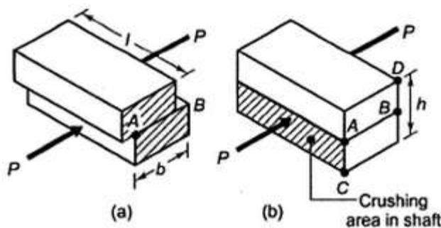
Figure 9 Forces Acting on Key Figure 10 Failure of Key a. Shear Failure b. Crushing Failure
