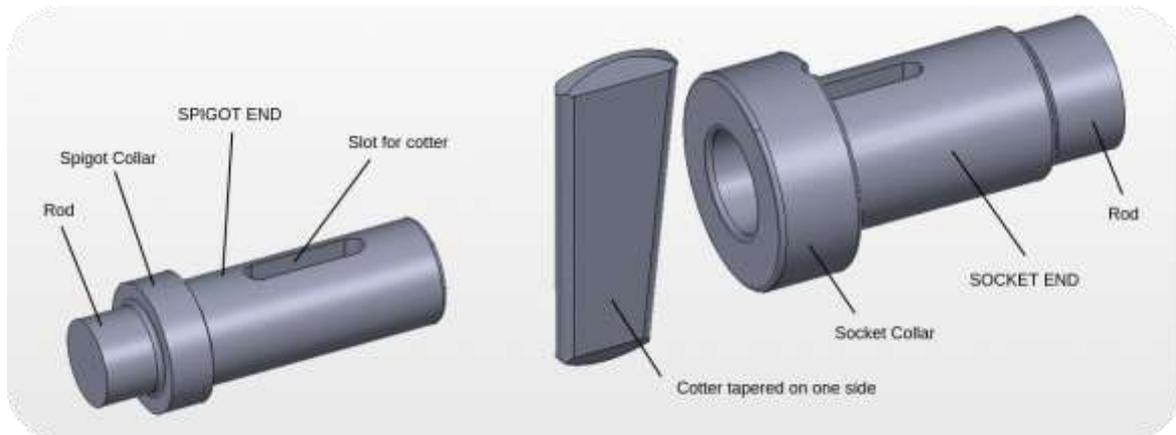
Exploded View of Cotter joint assembly
