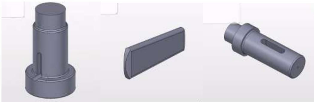
**Spigot** is the male part of the joint, it has a rectangular slot for passing the cotter through it. Spigot has a collar which rests against the socket end.
