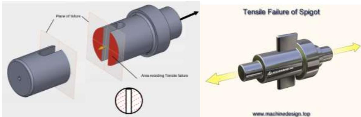
the area resisting the failure is shown by red in the diagram, since it is circular minus a rectangle the equation will be,
