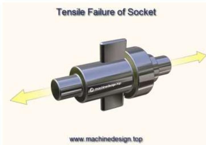
Area resisting is a hollow square minus a rectangular strip having length  $(d_1-d_2)$  and thickness  $t$ , so the strength equation becomes,
